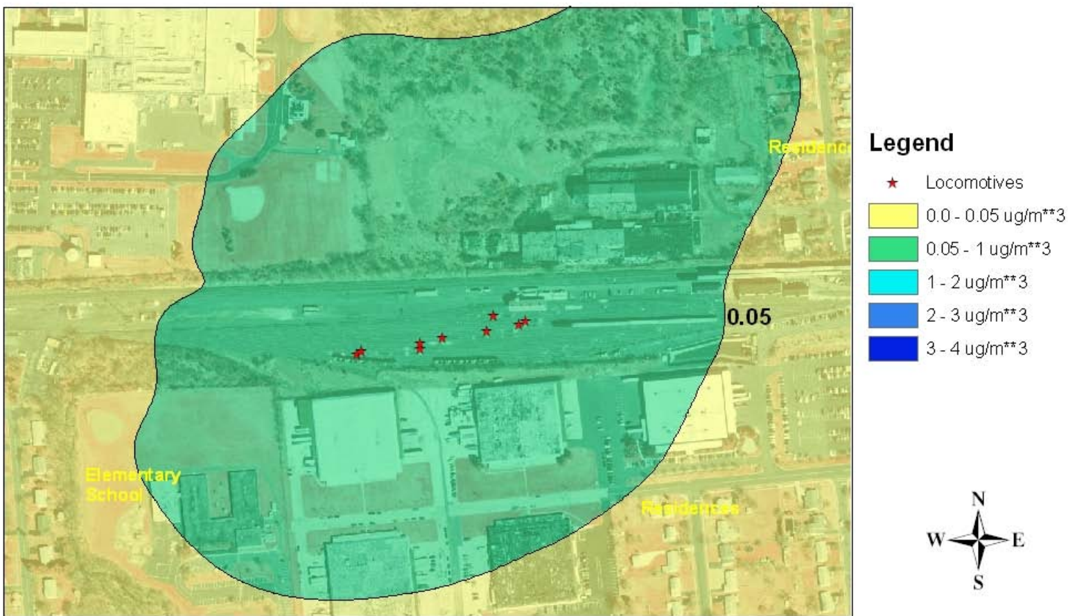
FIGURE 2: MAXIMUM PREDICTED ANNUAL PM2.5 CONCENTRATIONS: MAXIMUM 1 HOUR IDLING WHEN TEMPERATURES ARE ABOVE 0 deg.F, BASED ON NEW IDLING PROGRAM
